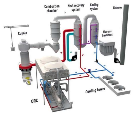
Figure 1: Schematic illustration of the Orchid solution for the use of waste heat for electricity generation (Graphics: Enertime)
